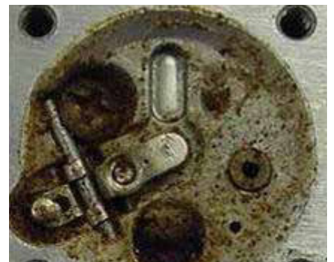
Carburetor damage from stale fuel
