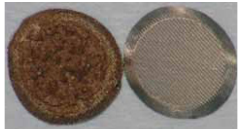
Left: Plugged fuel filter screen
