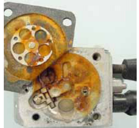
Corrosion from water inside carburetor
