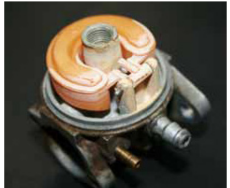
Corrosion inside carburetor
